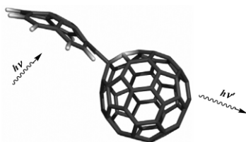
Fig. 1 Schematic representation of the unidirectional transduction of photonic energy from a parabolic corannulene antenna to the heterofullerene C 59 N.
